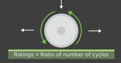
Using a circular blade that moves back- and-forth and under a fixed load of 500 grams, the Coup test machine measures the ratio of the number of cycles required to cut through the test sample vs. the reference material.
