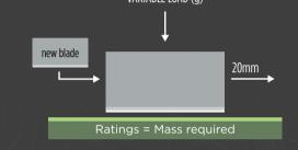
The Tomodynamometer (TDM-100) is used to determine the load required to cut through a glove sample using a straight-edge blade that moves along a straight path within a distance of 20mm. The sample is cut 5x each at three different loads
